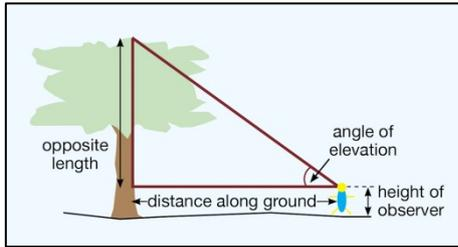
Record distance along the ground and angle of elevation in the field
